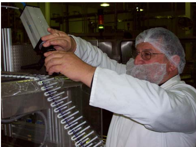
David Adermann installing a high speed video camera onto the production line
